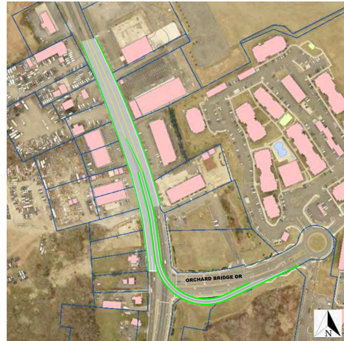
Figure 12: Option 4A Flyover at Orchard Bridge
