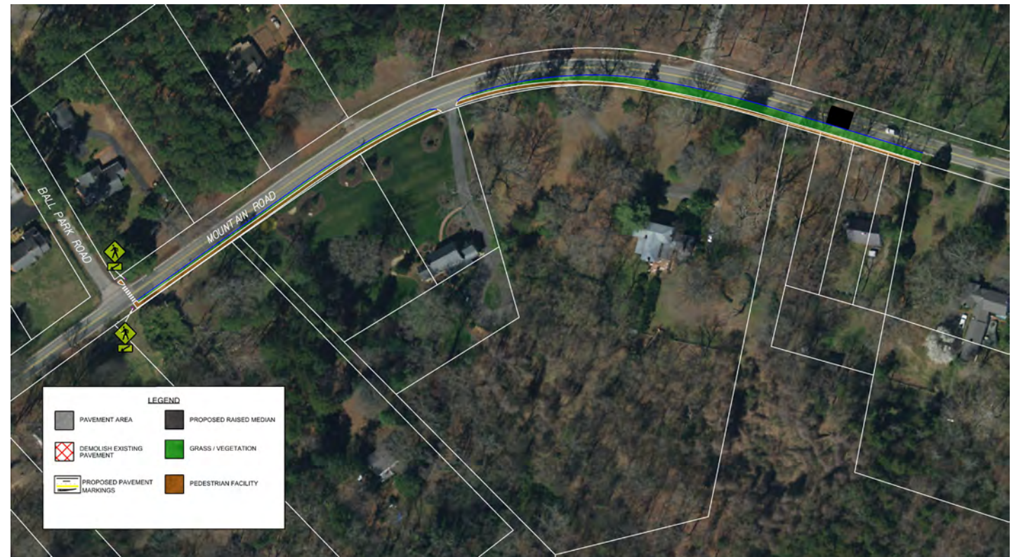
Figure 30. Mountain Road Sidewalk Improvements Concept C
