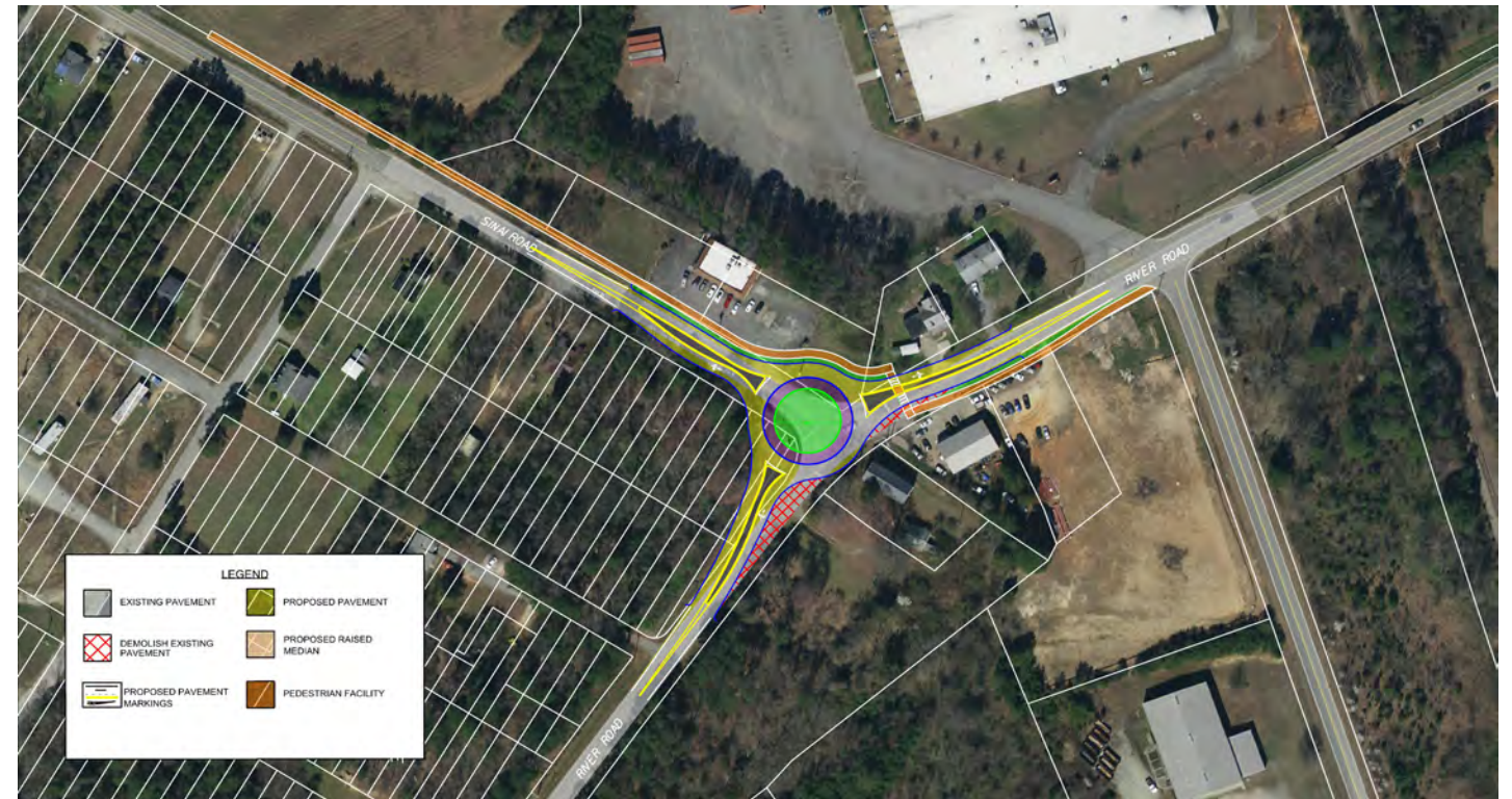
Figure 25. Mountain Rd at Sinai Rd Roundabout Concept
